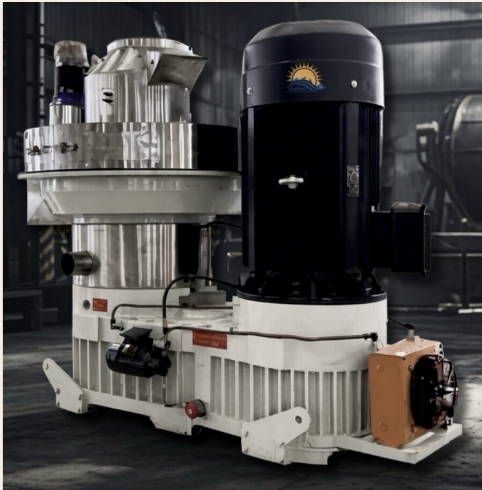
160 kW ring-die pellet mill · Sambalpur, Odisha
